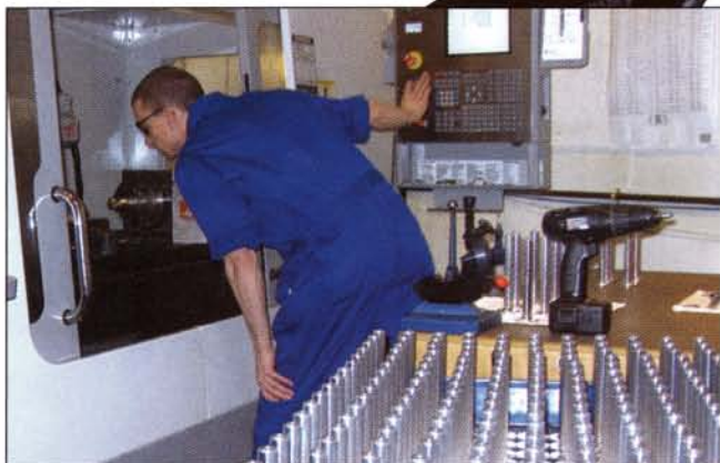
Raw materials ready to be fed into a Haas CNC HMC.
